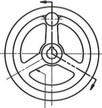
Spoke A omitted in the "preferred" section view
